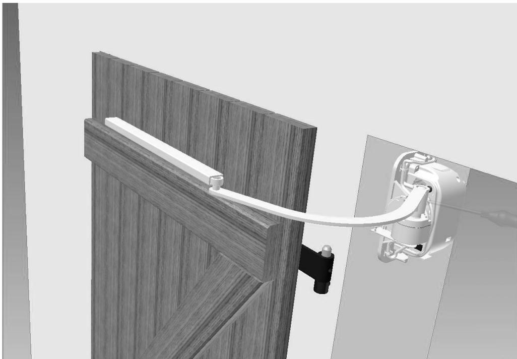
Monter les 2 embouts
